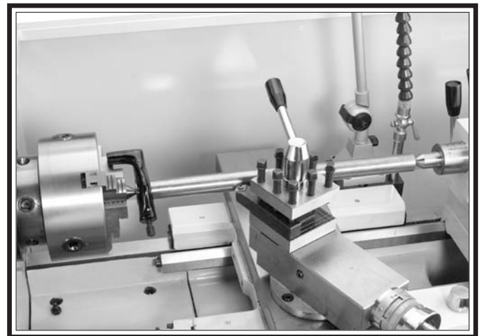
Figure 53. Example photo of stock mounted between the centers.
